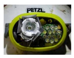
Next, gently lay the wires from the bulb base so they run towards the lower edge of the Duo headset and place the Solo into the headset, making sure the circuit board is towards the bottom of the headset.
