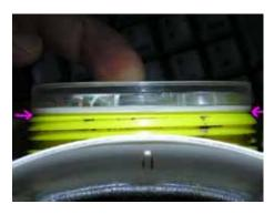
Next, carefully place the front lens on the front of the Duo, and make sure it seats properly. If not, adjust the position of the Solo until the lens does seat properly. The lens should lie flat, as indicated by a consistent small gap all round the edge (where the arrows are pointing
