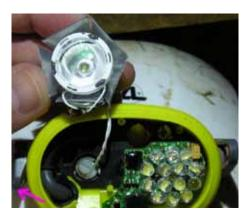
Turn the focussing lever 'up' to pull the bulb holder forwards.
