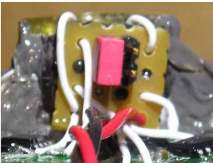
On the back of the R3 unit is a small board with some protruding pins and a small 'jumper' (seen as a red object in the picture). This jumper is used to control beam blending on the R3.
