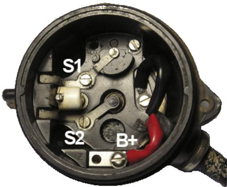
Next, connect the (black) switch input leads, each to one switch contact (S1 and S2). It does not matter which black wire connects to which switch contact.
